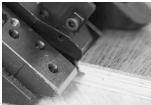
Fig. 13 Pushed in to the groove = correct position
